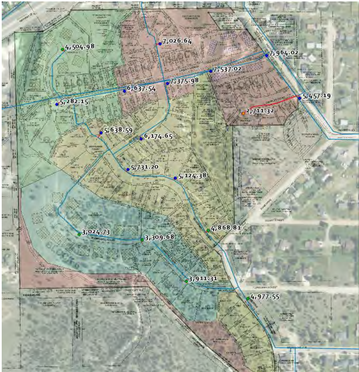
Figure 4 Hydrant Available Flowrates for Fire flow Analysis
