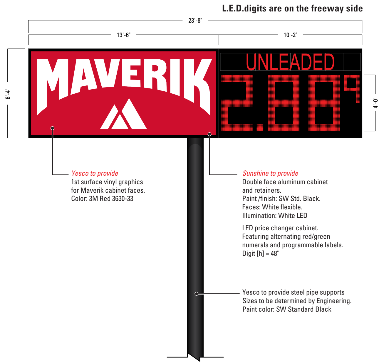
1.0 DOUBLE FACE HIGH-RISE POLE SIGN (DETAIL) TOTAL SIGN AREA = 120 FT 2 SCALE: 1/4" = 1'-0"
